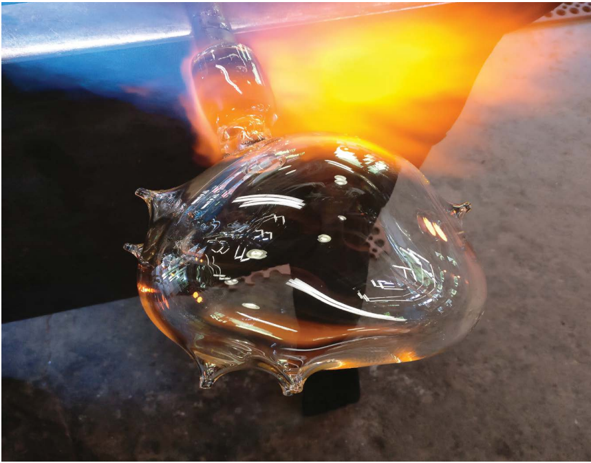
Fig. 5. Spikes are added by pulling heated parts from the glass surface. These node points are clearly identifiable in the 3D scan. They are geometric interface points for the 3D printing, Glass Mutations . (© 2017 Tobias Klein)
