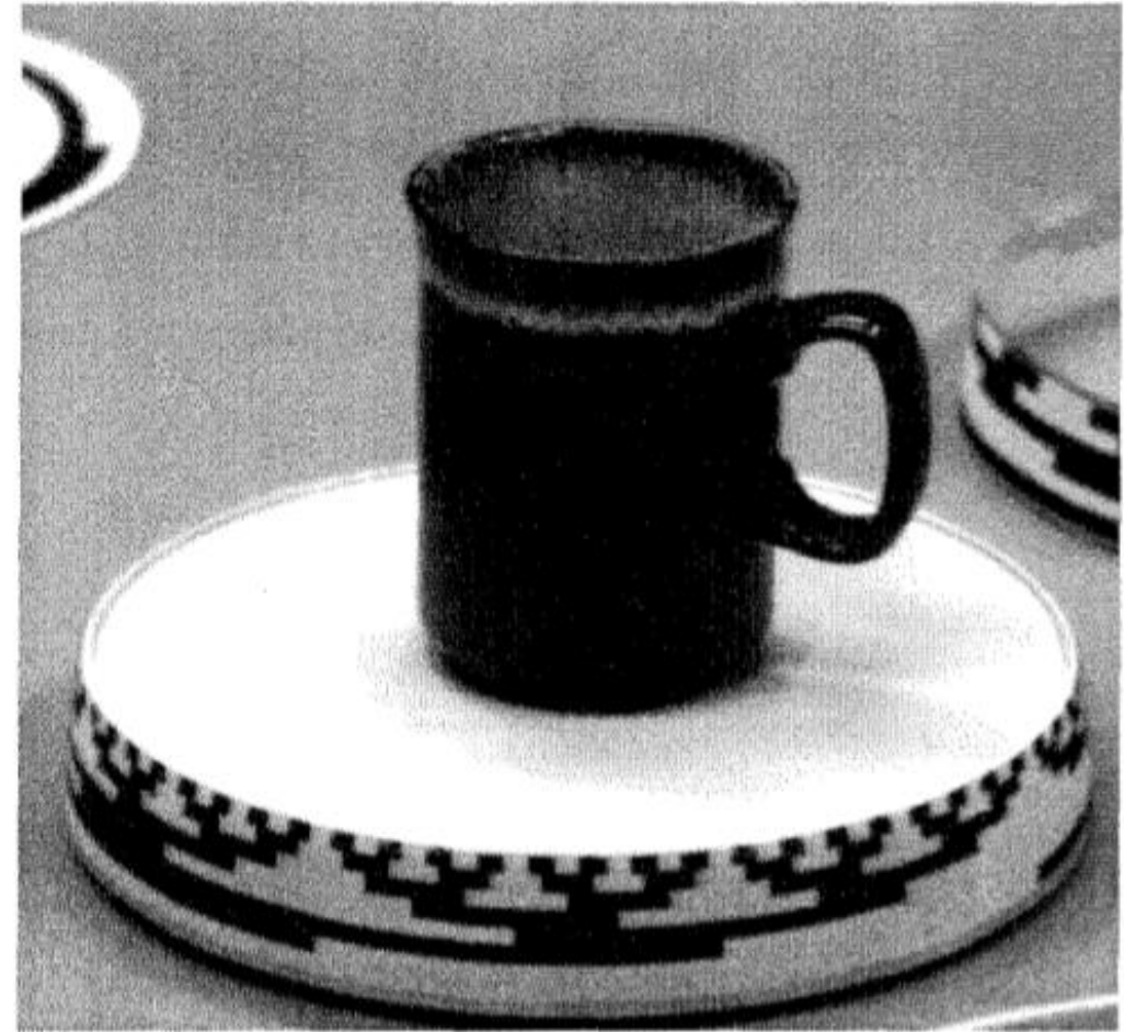
FIG. 6. Input image of object (cup), turntable, and position coding ring.
