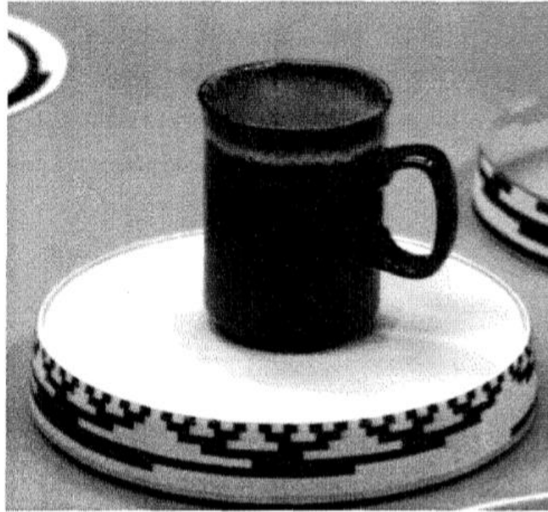
FIG. 6. Input image of object (cup), turntable, and position coding ring.
